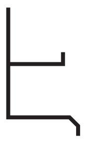
Provides a plaster stop/drip molding with an aesthetic reveal for window heads, tops of door frames and plate conditions where a drip edge is required.
