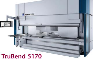
14ft 170 ton TruBend 5170 press brake is capable of bending thin & thick complex sheet metal parts with high levels of angular accuracy. Features such as lower tool displacement for hemming and 6 axis backguages provide us a unique advantage and complete production freedom from programming, to set up, to bending productivity the innovated features of this machine allow us to be
