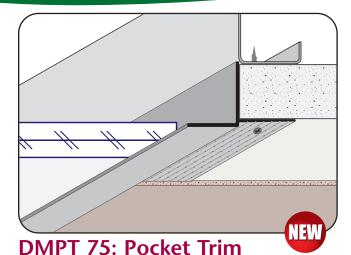
• Available in Aluminum Alloy (6063 T-5) The DMPT Pocket Trim provides a smooth, in-plane transition between a drywall ceiling and an acoustical ceiling, and supports the acoustical ceiling tile. Key holes on the taping flange help key the drywall mud to the Pocket Trim.
