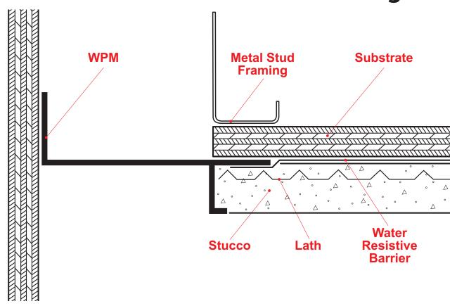
A screed that provides a plaster stop and creates a reveal at ceiling/wall conditions. Vented to provide free air flow at the perimeter.
