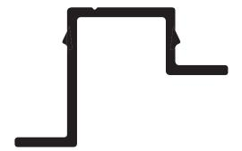
The VO-FCP Vertical Offset Insert creates an attractive 1/2" architectural reveal when used in conjunction with the VR-FCP Vertical Retainer (sold separately). This is an excellent molding for the transition from a single layer of fiber cement panels to overlapping siding.
