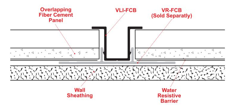
The VLI-FCP Vertical Lap Insert creates an architectural 1/2" reveal when used with the VR-FCP Vertical Retainer (sold separately).
