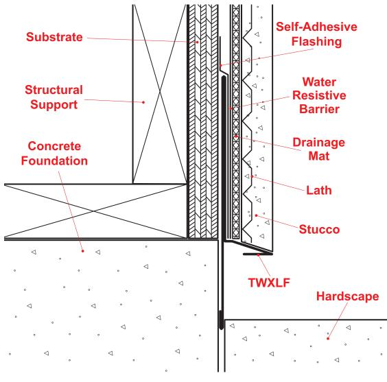
Stucco installation guidelines require stucco to be held up off the hardscape 2". The TWXLF provides weep slots in line with the drainage mat to maximize the drainage and ventilation per 2021 IBC: 2510.6.1
