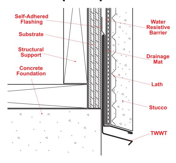
The Tru-Weep™ Weep Screed is a single piece counter flashing stucco weep screed specifically designed to be used with drainage mat. Weep slots are located along the back of the sloped leg in alignment with the drainage mat to allow water to efficiently exit the stucco assembly.
