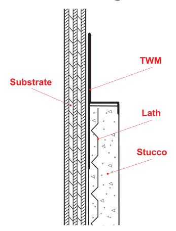
One-piece SolidGround<sup>®</sup> design feature mitigates the concern of moisture penetration in a horizontal condition.Provides a plaster stop for top of wall/parapet conditions. SolidGround<sup>®</sup> design prevents moisture penetration at the top of the wall.
