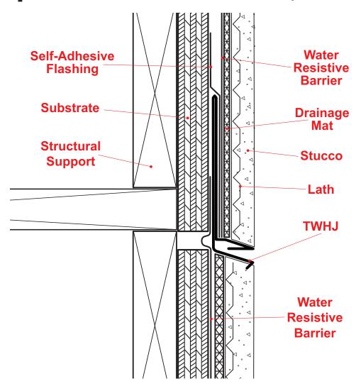
The Tru-Weep™ Horizontal Control Joint is a single piece horizontal control joint specifically designed to be used with drainage mat. Weep slots are located along the back of the sloped leg in alignment with the drainage mat to allow water to efficiently exit the stucco assembly.
