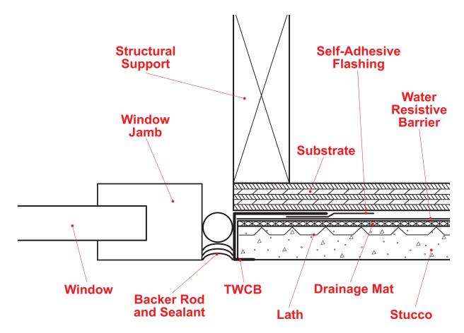
The Tru-Weep<sup>™</sup> Casing Bead is a non-perforated customizable stucco casing bead. Whether the stucco assembly is utilizing a drainage mat, continuous insulation, or traditional 3-coat the Tru-Weep<sup>™</sup> Window Jamb can be ordered in any ground size to accommodate the stucco assembly.
