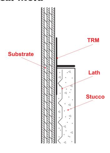
One-piece SolidGround® design feature mitigates the concern of moisture penetration in a horizontal condition. Provides a reveal and plaster stop at parapet top and function as a depth screed. Can be used at ceiling to wall conditions when dealing with dissimilar materials.
