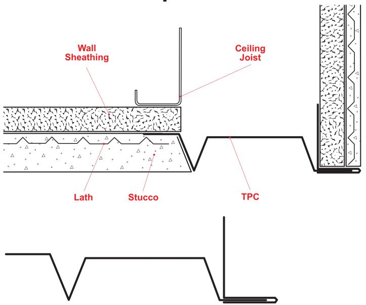
A functional two piece product specifically designed for the fascia/soffit corner that provides a reveal and allows movement at this condition.
