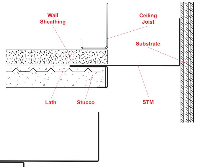
Provides a decorative transition between ceiling/wall with return keys for screeding of plaster. Can be vented for perimeter airflow into space above.
