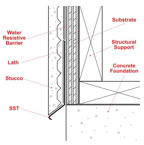
A variation of the traditional weep screed that provides a plaster stop and weep function at the foundation line.
