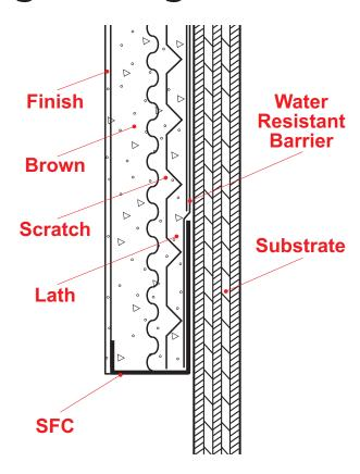
This is the most frequently used casing bead for terminating drywall and plaster.
