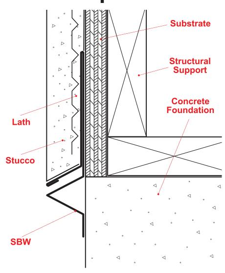
A unique one piece weep screed design that combines the features of a traditional foundation weep screed while providing an aesthetically pleasing look. The upper leg has a plaster stop with a 1/4" closed hem for safety and weep holes.
