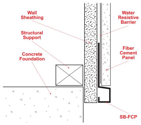
A functional starter trim piece for the fiber cement panel that also provides a weep point for moisture.
