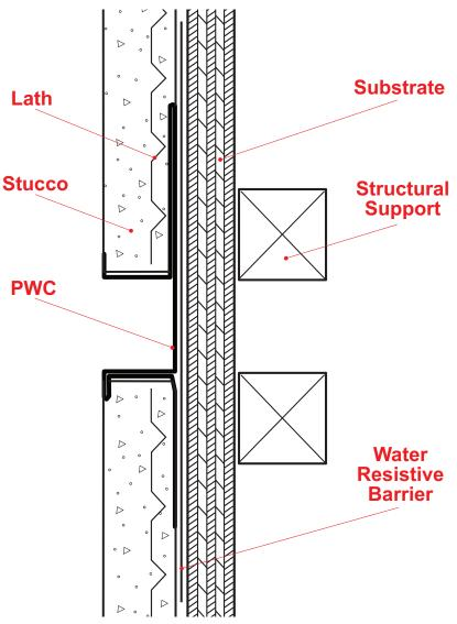
One-piece SolidGround<sup>®</sup> design feature mitigates the concern of moisture penetration in a horizontal condition.
