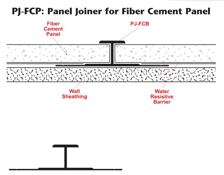
A functional trim piece used to join two panels together in a vertical condition.
