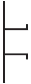
A decorative reveal used as a plaster stop/control screed for conventional 3-coat stucco to separate dissimilar materials and/or to create aesthetically pleasing shadow lines on the exterior walls, ceilings and soffits.
