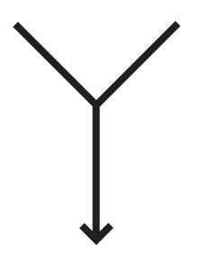
Creates a plaster stop and high strength corner for conventional 3-coat stucco with an aesthetically pleasing exposed edge at all outside corner conditions.
