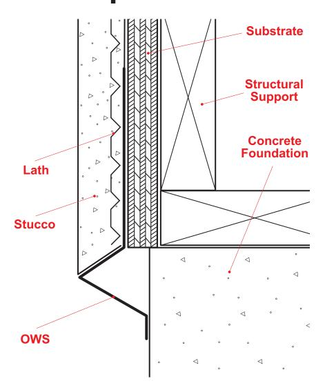
A special weep screed for those conditions where the sheer wall exceeds the foundation in plane. This special design permits the bottom leg of the weep screed to return back to the foundation. Avaiable with dual weep holes to allow full passthrough of moister.
