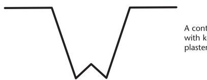
A control joint with a minimal reveal. Available with key holes in the nailing flange for better plaster adhesion.
