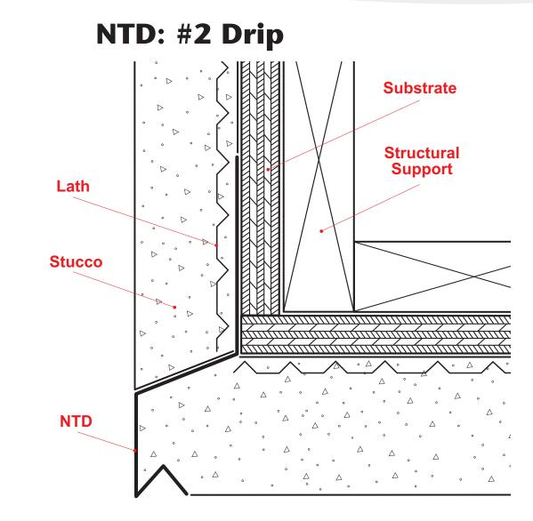
A plaster drip screed that helps align the soffit to give it a clean, straight edge at the fascia/soffit line. Provides a unique 3/4" "flush" reveal at the fascia.
