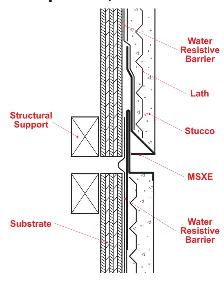
Econo M-Slide Expansion Joint® is a version of the M-Slide Expansion Joint® product line that does not have the additional back leg behind the sloped screed along the upper portion of the profile. The dual function self-aligning expansion joint provides movement capability at floor line while allowing moisture to release from the top ground and lock out moisture from the bottom.
