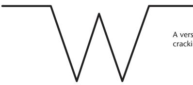
A versatile control joint used primarily to relieve cracking. Provides a decorative reveal.
