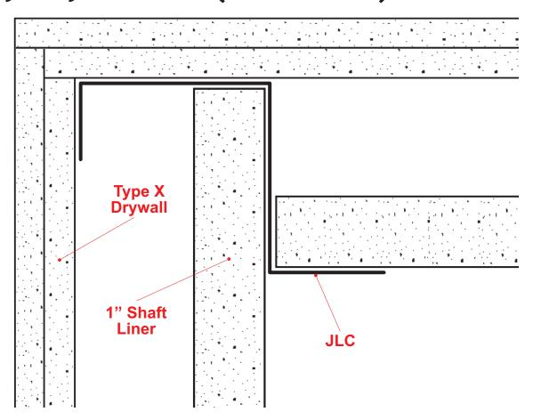
Stockton Products JL Corner is single piece metal framing member designed for outside corners within shaft wall assemblies.
