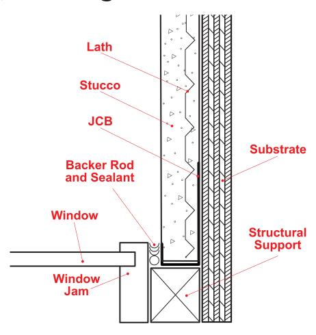
Standard plaster stop/casing bead for terminating stucco with an extended return key for caulking.
