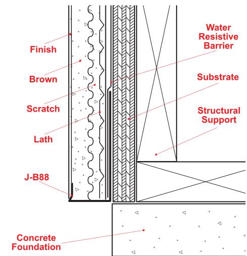
Similar to the new SFC88 Short Flange "Finish Rite<sup>®</sup>" plaster trim, the J-B88 Long Flange J bead provides all the same features of controlling the brown coat thickness, but has a 3 1/2" nail flange and 1/2" diameter weep holes for those conditions where a weep function is required.
