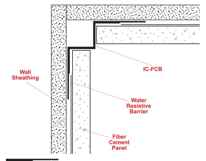
Used in an inside corner condition where two Fiber Cement Panels meet.
