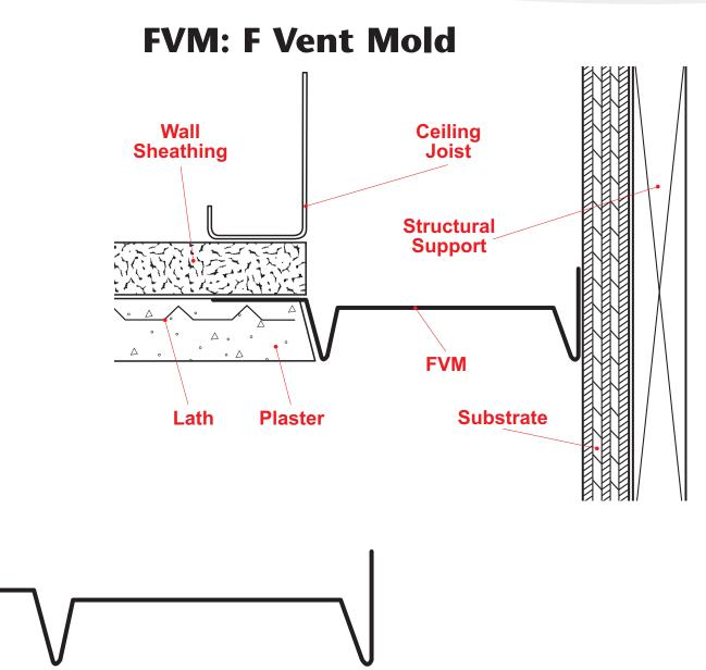
The F Vent Mold is designed to butt against walls on one side with an extended attachment flange providing perimeter airflow. Available non-vented for use as a decorative reveal.
