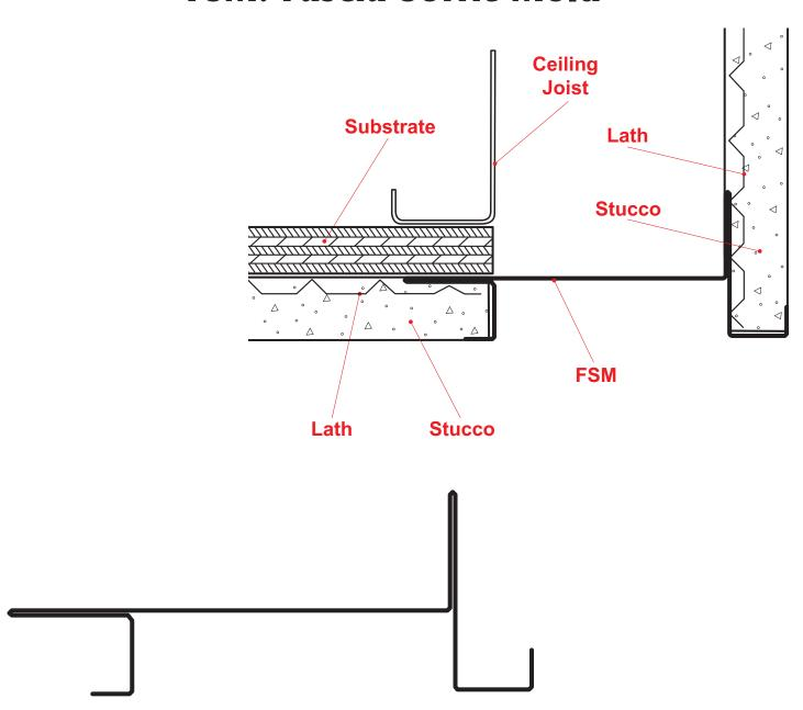
Creates a decorative reveal at fascia/soffit transition providing a small overhang drip edge. Has return keys for screeding of stucco. Extended attachment flanges provides area to overlay lathing. Can be vented for perimeter airflow into space above.
