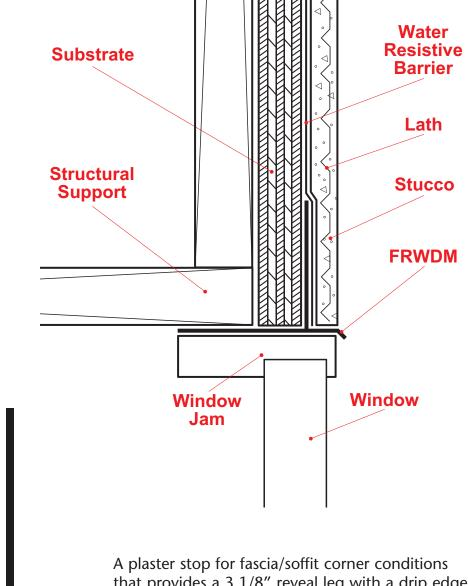
that provides a 3 1/8" reveal leg with a drip edge for recessed window conditions where a drip edge is required. Can also be used when a caulking leg is required for backer rod and sealant.
