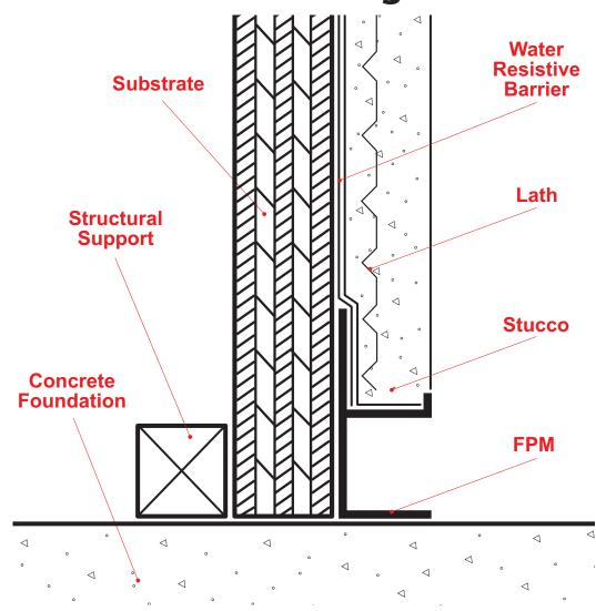
A plaster stop/control screed for conventional 3-coat stucco, used at the top or base of columns, the top of walls at the ceiling, or at the base to create a reveal. Also used at the top of windows to permit the continuation of a horizontal reveal at the window line.
