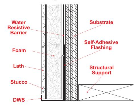
The Slotted Weep Screed is a single piece weep screed specifically designed provide a route for moisture to escape. Weep slots are located along the back of the weep screed allow moisture to efficiently exit the stucco assembly.
