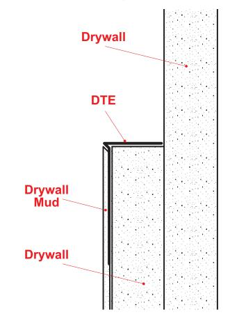
Creates a protective and decorative edge for drywall at any termination point. Includes key holes for drywall mud adhesion.
