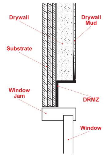
The Z Wall Reveal hash a taping flange that provides a reveal and a termination point for drywall at door frames, windows and wall bases. Includes key holes for drywall vent slots in the reveal.
