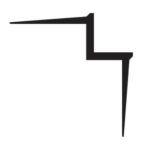
"W" style drywall molding with taping flanges that creates an inverted corner for setbacks, stepdowns and other special drywall conditions. Includes key holes for drywall mud adhesion.
