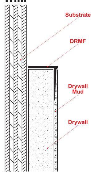
"L" style drywall molding with a taping flange that provides a drywall termination point by capping of the raw edge of the drywall board. Includes key holes for drywall mud adhesion.
