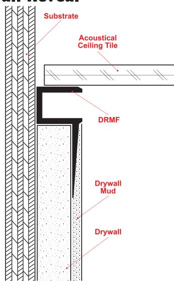
"F" style with a taping flange that creates a reveal and board termination point at tops and bases of walls, and at door and window frames. Includes key holes for drywall mud adhesion.
