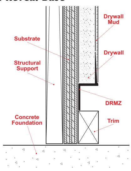
These "Z" style Reveal Base has a taping flange that provides a reveal and a termination point for drywall in a base condition. Includes key holes for drywall mud adhesion.
