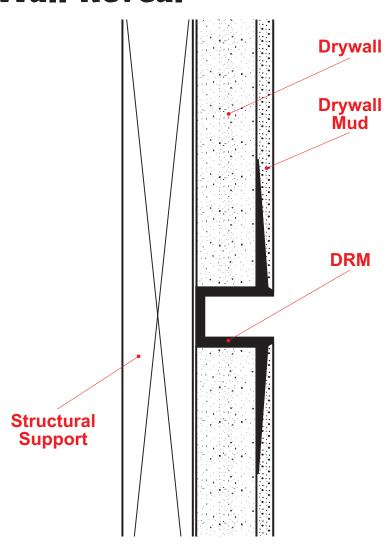
A reveal molding with taping flanges that provides a decorative reveal in drywall. This molding is installed after the drywall board, greatly improving installation ease and time. Includes key holes for drywall mud adhesion.
