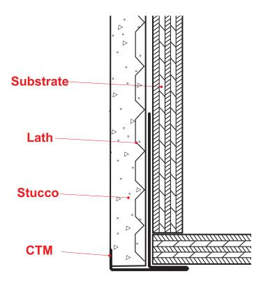
A plaster stop used in various applications to finish an edge or bridge when using dissimilar materials. Can be used to support acoustical tile or to case off windows.
