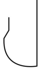
A drywall stop/casing bead in a bullnose shape that provides a decorative casing around windows, doors, and at the base of walls. Keyholes in the tape flange help the drywall mud key to the trim piece.
