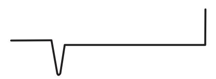
Provides a ventilated finish at the juncture of soffit and fascia providing attachment by a wing in attic. Available non-vented for use as a decorative reveal upon request.
