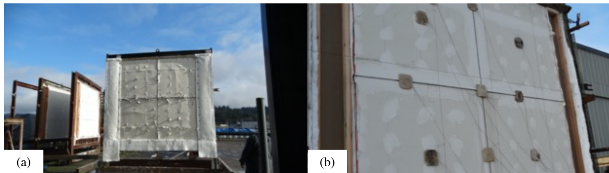
Figure 8. Wall assembly showing (a) after furnace and (b) after test – unexposed.
