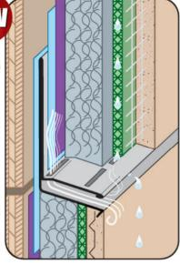
The Tru-Weep™ Stucco Accessories are a series of counter flashing stucco screeds specifically designed to be used with drainage mats and (CI) continuous insulation. Weep slots are located along the back of the sloped leg in alignment with the drainage mat to allow water to exit the stucco assembly efficiently.
