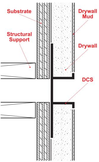
Drywall version of the plaster channel screed used to create a decorative reveal and to separate dissimilar materials if desired. Used with one-coat stucco and direct applied systems. Available with 1/8" weep holes.
